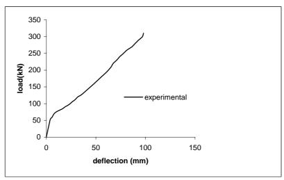
Fig 3 Load-deflection curve for control beam
