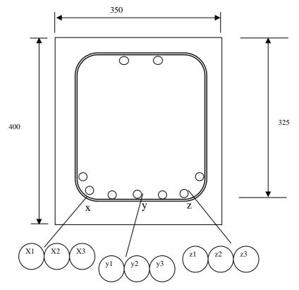
Fig 5 Specimen configuration and measurement points of temperature at the rebars
