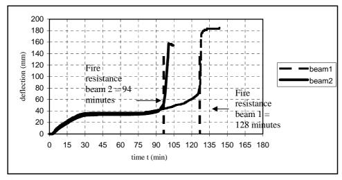
Fig 7 Heating time-deflection curves for beam 1 and beam 2
