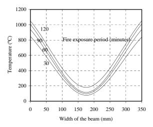
**Fig 10** Temperature profile in the cross section of the beam 1 80mm from bottom of the beam for different fire exposure periods. The temperature of each side of the beam is an average reading from TC's in furnace on the each side of the beam.
