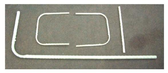
Fig 1a GFRP rebar shapes used as reinforcement for control beam and beam 1
