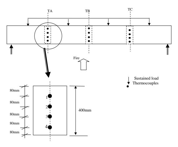
**Fig 4** Thermocouples embedded in concrete. Group of thermocouples at A, B and C in concrete Nos. 1-4 at centre line 80mm c/c (3x4=12).
