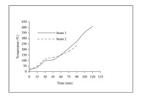
Fig 12 Average stirrups temperature in beam 1 and beam 2
