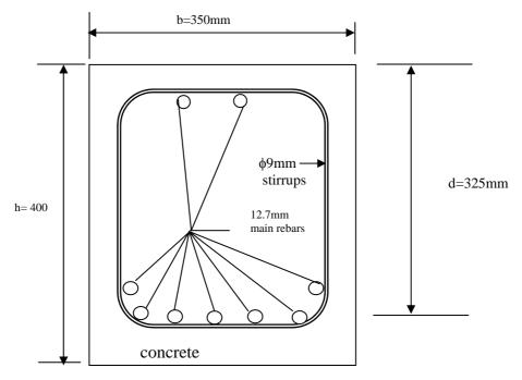
Fig 1b Beam cross section with reinforcement arrangement
