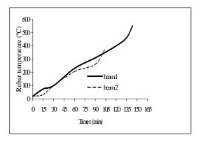
Fig 11 Heating time/ temperature in the rebars for beam1 and beam 2
