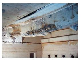
Fig 9 Failure of beam 2 after fire test inside the furnace shows some flexural cracks and rupture in the main reinforcement
