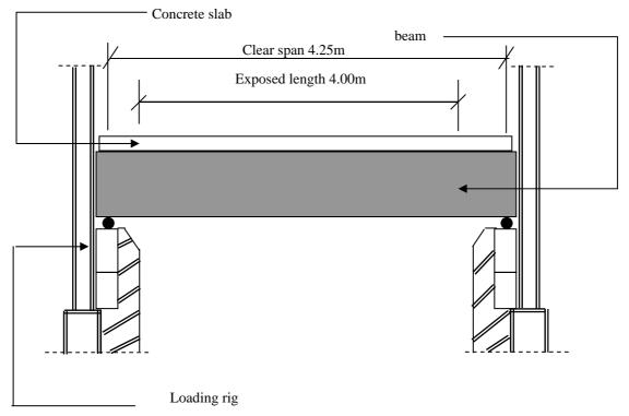
Fig 6 Fire test set up
