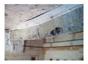
**Fig 8** Rupture at the mid centre of the concrete in beam 1 after fire test
