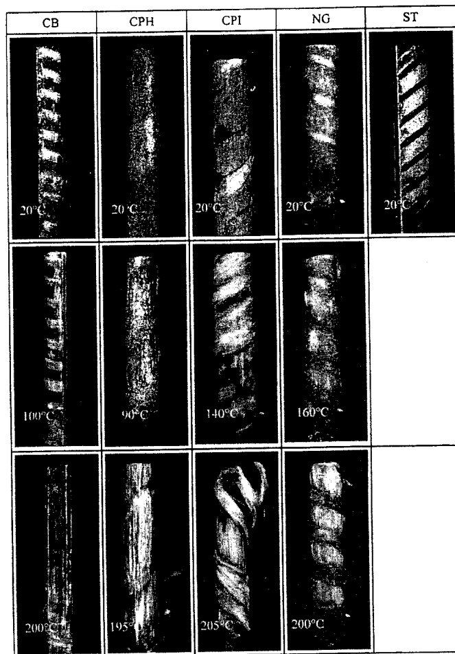
FIG. 9. Images of FRP Rebars after Pullout at Different Temperatures
