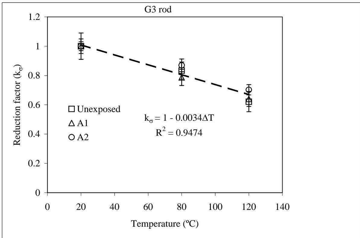
**Fig 13** Temperature dependent tensile strength of G3 rod
