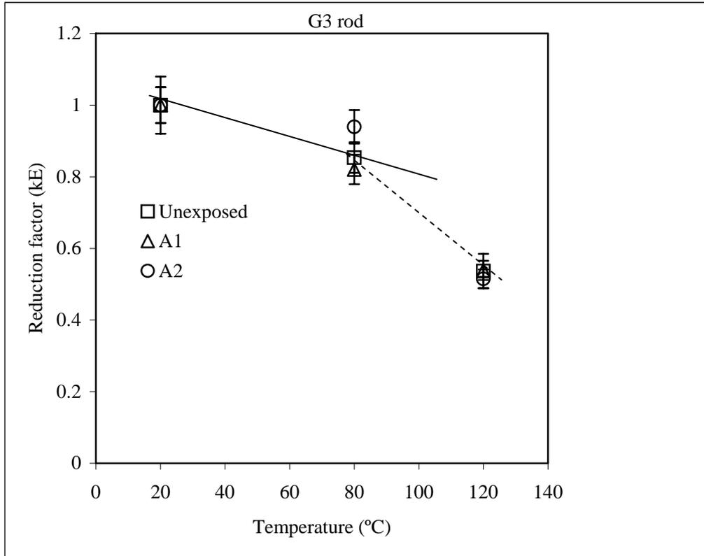
**Fig 16** Temperature dependent elastic modulus of G3 rod
