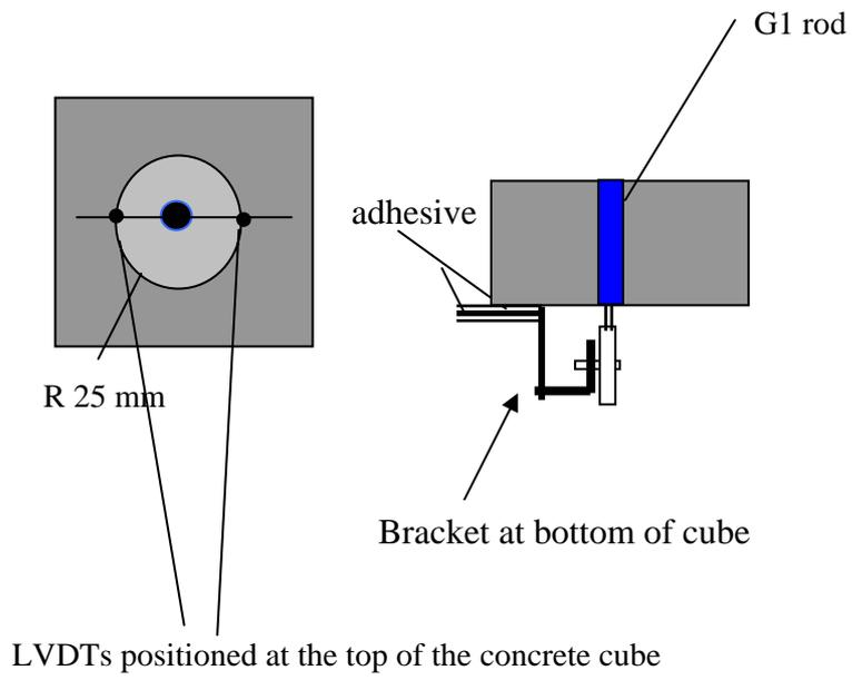
**Fig 3.** Relative movement points of the GFRP rebar in the pullout test
