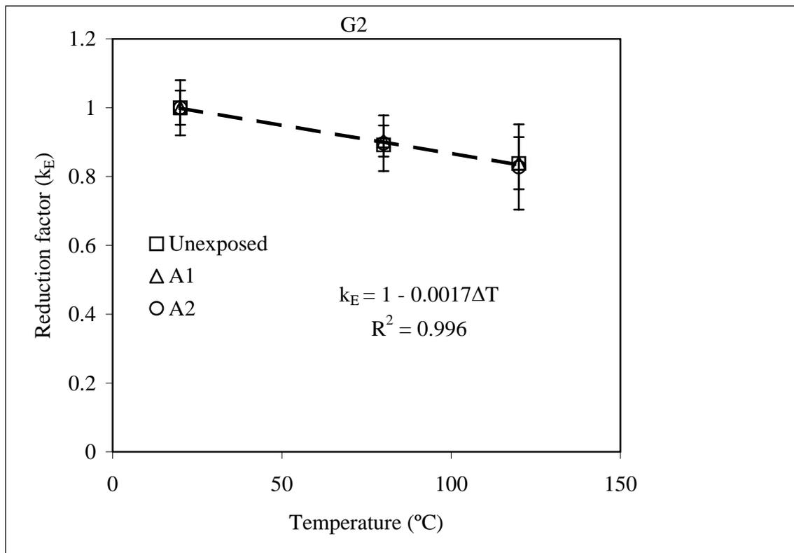
**Fig 15** Temperature dependent elastic modulus of G2 rod
