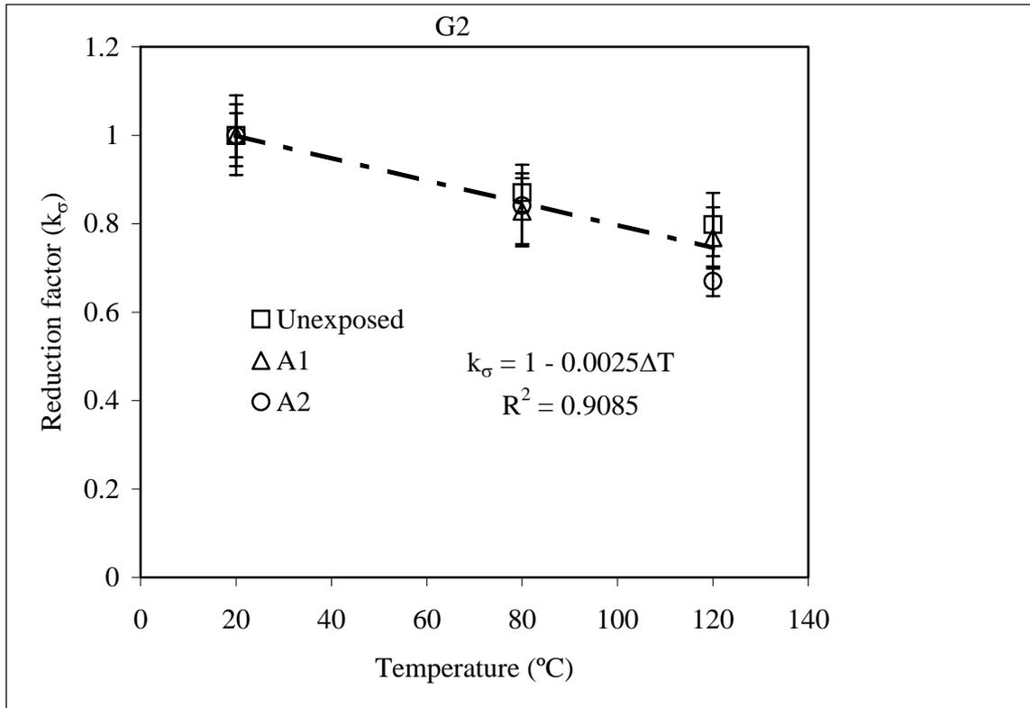
**Fig 12** Temperature dependent tensile strength of G2 rod
