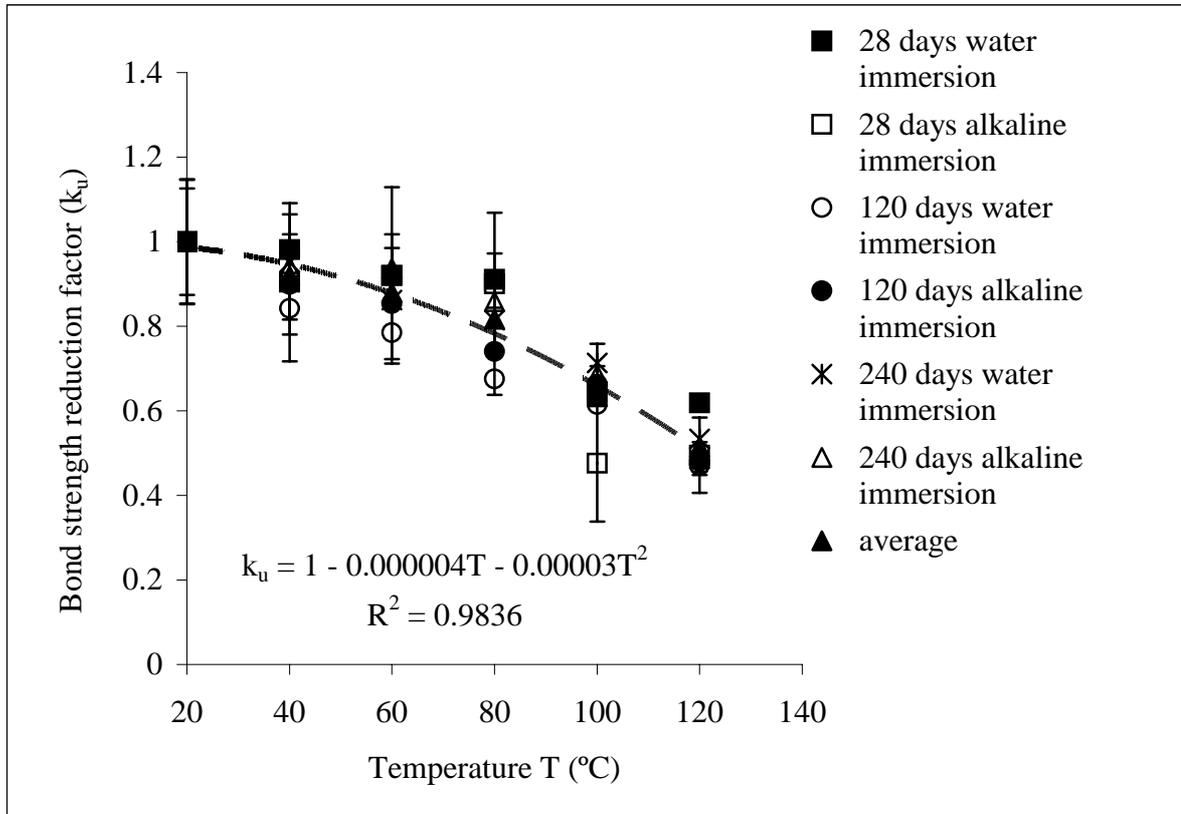
**Fig 7** The relationship between the bond strength reduction factor and temperature. The reduction factor is calculated for each environmental conditioning regime and is based on the strength of the bond at a given temperature, relative to the strength at room temperature after that specific environmental treatment.
