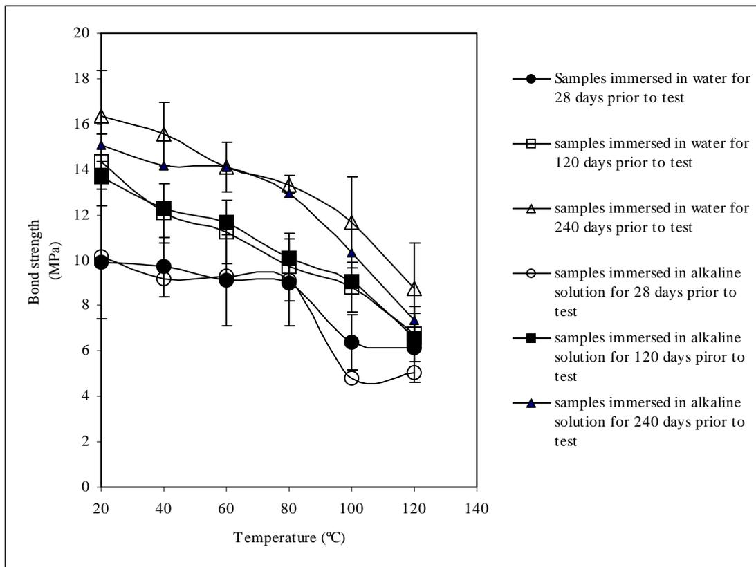
**Fig 6.** Comparison of pull - out test results for the composite rebar-concrete samples at differing temperatures and after various conditioning environments. The standard deviations shown are, for clarity, only for those samples exposed to water.
