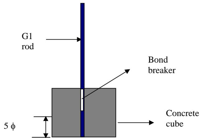
**Fig 2.** Pull - out test sample
