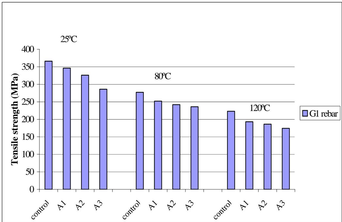
**Fig 10.** change in strength of G1 rod with different environment
