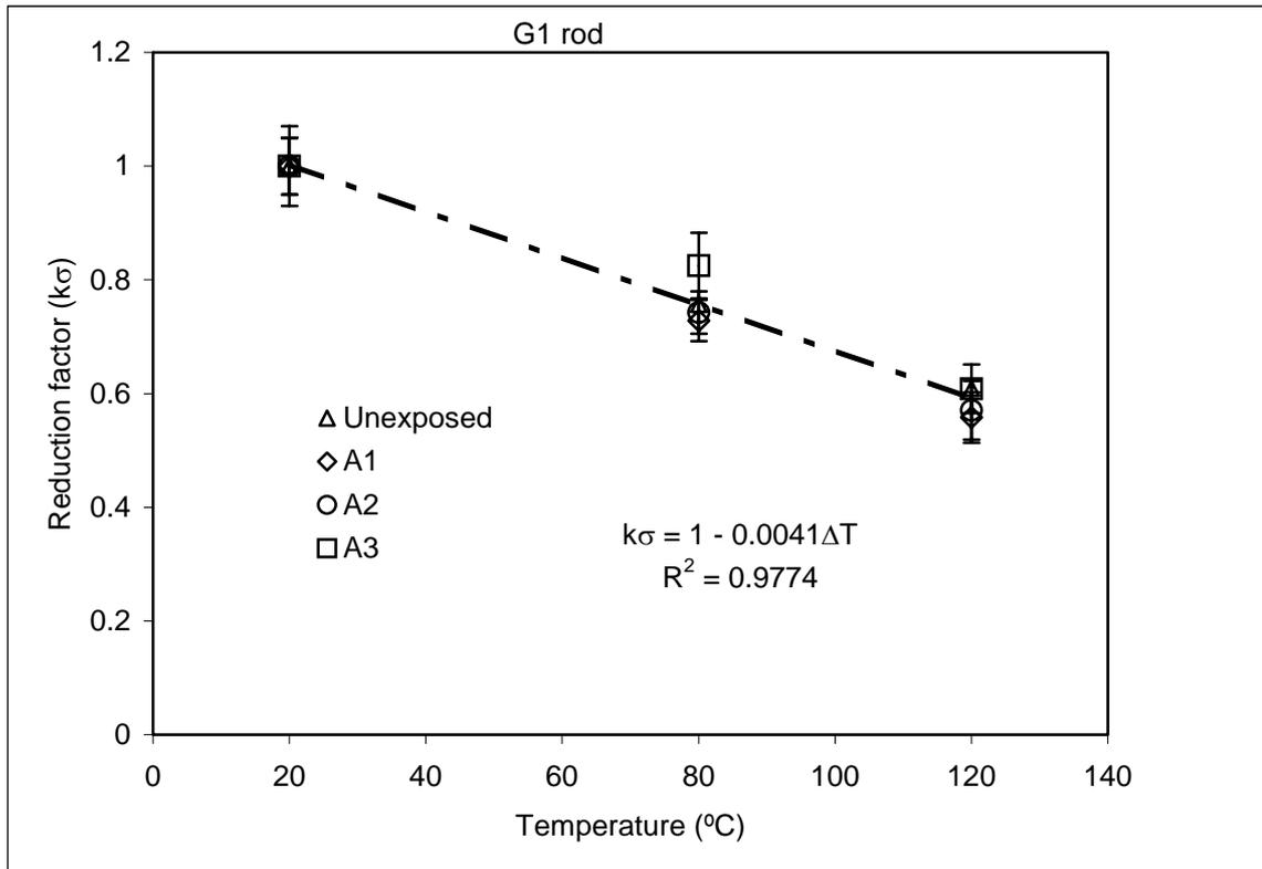
**Fig 11** Temperature dependent tensile strength of G1 rod
